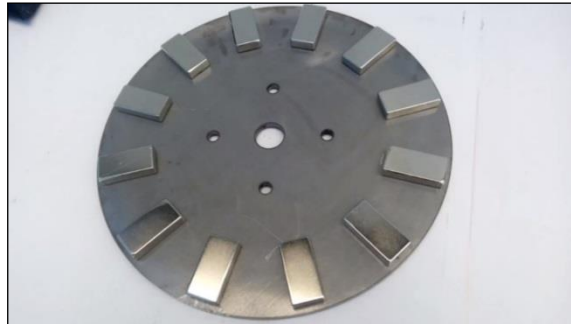
Figure 13. Picture of 12 Neodymium magnets attached to the rotor disc
